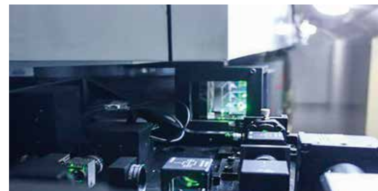
Platform attitude monitoring and adjustment equipment based on laser reference surface
