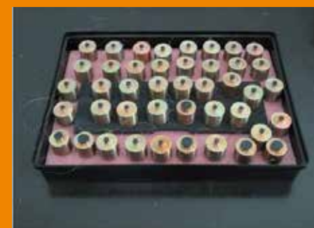
High temperature coating for heat flux transducer
