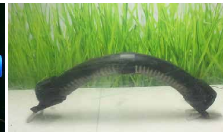
Inchworm-inspired soft crawling robot
