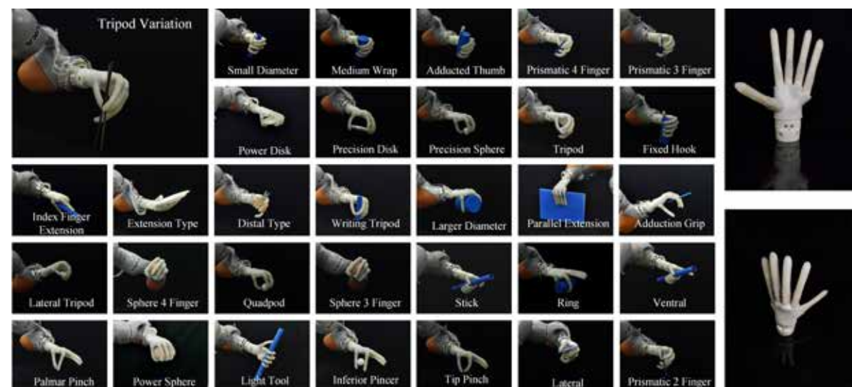
Rigid-soft humanoid dexterous hand and 32 grasp types
