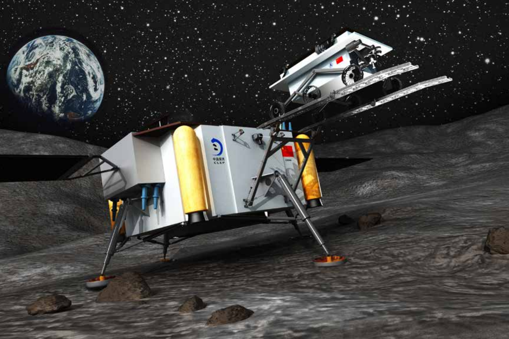
Movement and transfer mechanisms of China's Yutu lunar rover
