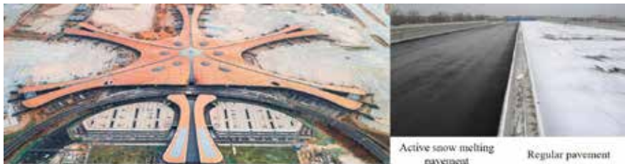
Application of active snow melting technology on pavement surface at Beijing Daxing Airport
