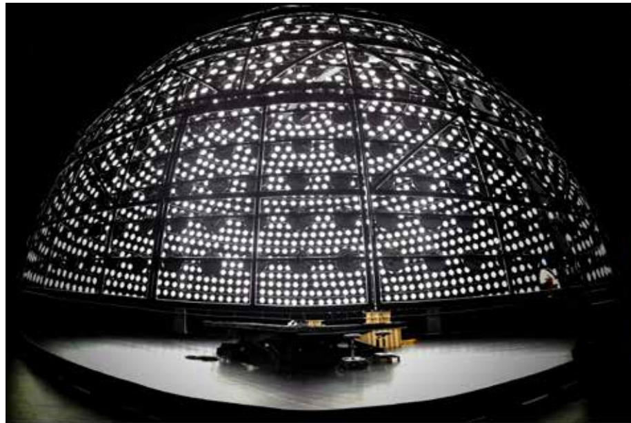
Daylight environment simulation based on artificial sky
